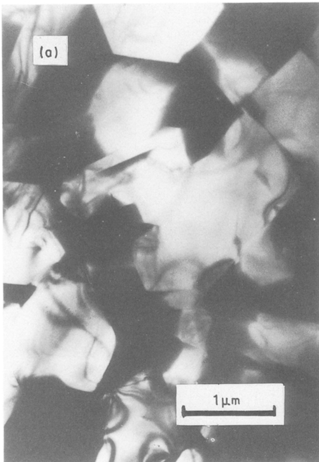
Figure 6 TEM of (a) \text{Si}_3\text{N}_4 with 10 mol % and (b) \text{Si}_3\text{N}_4 with 1 mol % of \text{Y}_2\text{O}_3\text{-Nd}_2\text{O}_3 sintered at 1900 °C for 4 h in 10 MPa \text{N}_2 .
